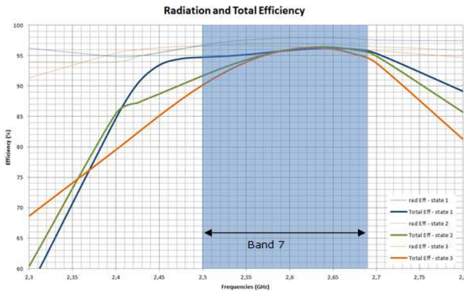
Figure 40 Radiation and total efficiency of the antenna system within the LTE band 7
